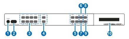
**1 POWER Button:** Press this button to power the unit on (green LED) or place it into stand-by mode (red LED).
