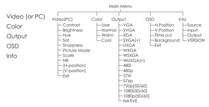
Use +, - button to move highlight bar to your desired parameter, then press MENU/ENTER to enter into sub-menu of your selected parameter.
