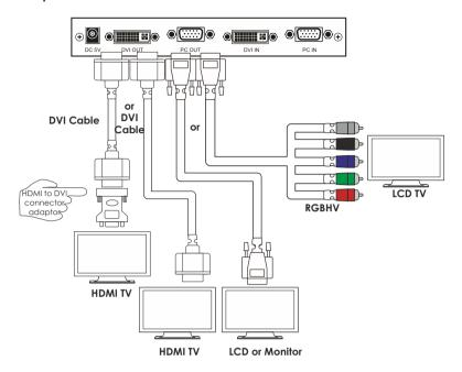
The device can output a variety of PC, SD and HD resolutions in both digital and analog format simultaneously. The digital output is available from the DVI output connector while the analog output is available from the PC D-sub output connector.
