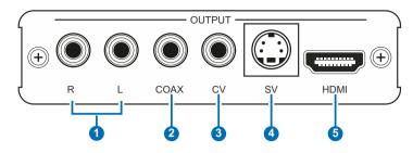
R/L OUTPUT: Connect to active speaker with RCA cables for sychronize video output with HDMI, S-Vide or Composite video.
