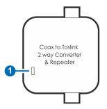
1 POWER LED: The LED will illuminate when the power is connected.
